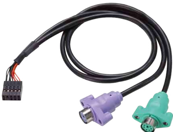
PS-2 Cable , 2*Mini Din 6p ( K.B & Mouse ) to 10p Housing
